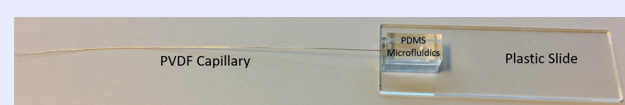
Figure 4 Microfluidic MS emitter for picodroplet analysis
